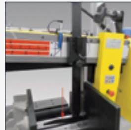
**TP:** Cilindro verticale per la chiusura a pacco. *Vertical cylinder for bundle cutting.*
